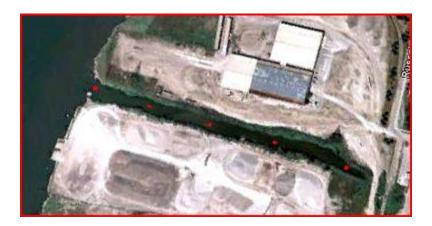
Basic water quality measurements were collected during each seasonal survey (Table 4). Temperature (°C), pH, conductivity ( $\mu$ S/cm), oxidation-reduction potential (mvolts), and dissolved oxygen (mg/L) were measured *in situ* using a Hydrolab Surveyor 3/ Reporter Multiprobe Multiparameter Water Quality Logging System. Measurements were collected approximately 50 cm below the surface.
