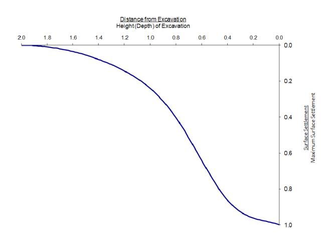
GROUND SURFACE DISPLACEMENTS FROM CUT AND COVER EXCAVATIONS
