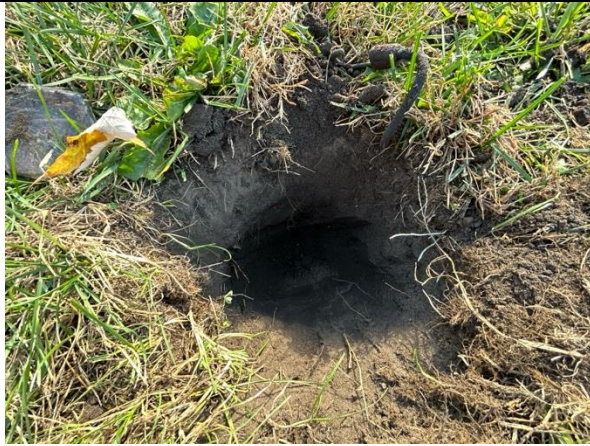
IMAGE 3 EXCAVATED TEST PIT
