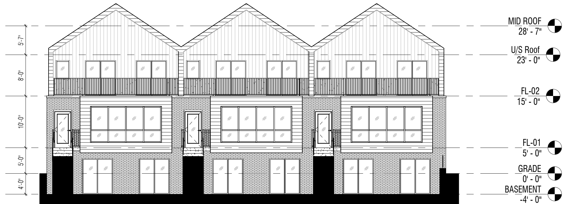
1 NORTH ELEVATION SK5 3/32" = 1'-0"
