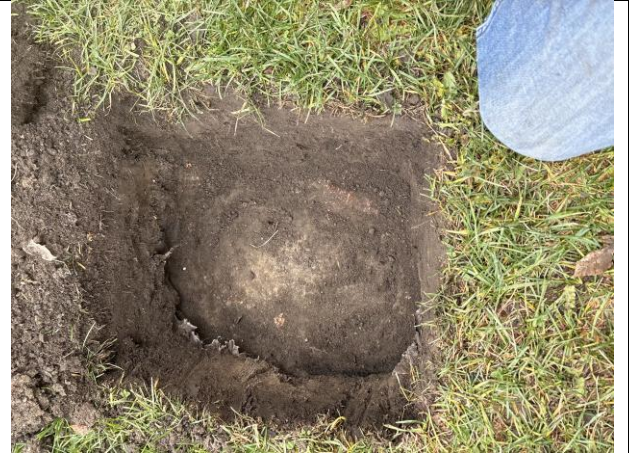
IMAGE 6 EXCAVATED TEST PIT, ABOUT 50CM DEEP
