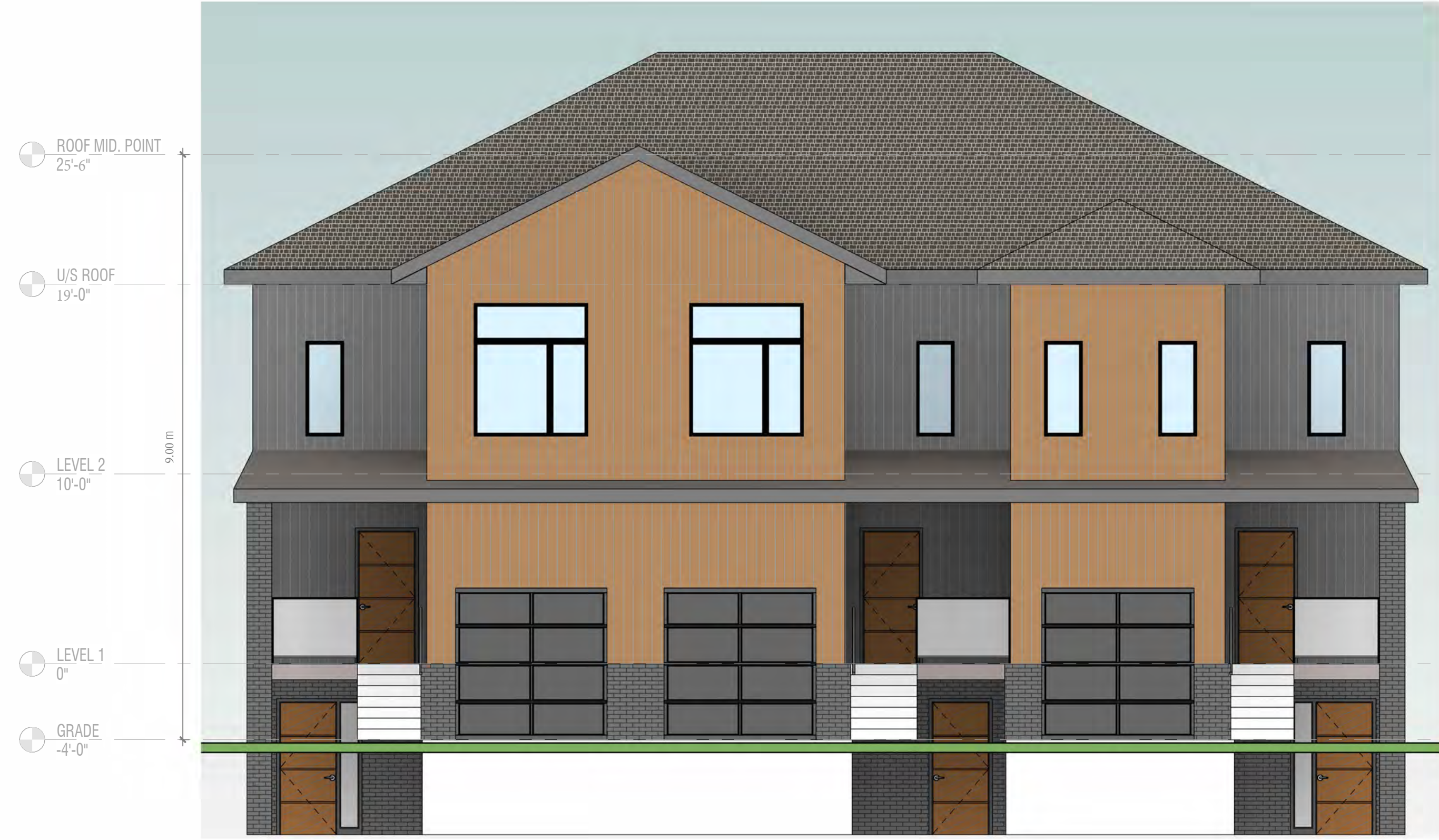
4 3 BLOCK T.H. - FRONT ELEVATION SCM-3 3/16" = 1'-0"
