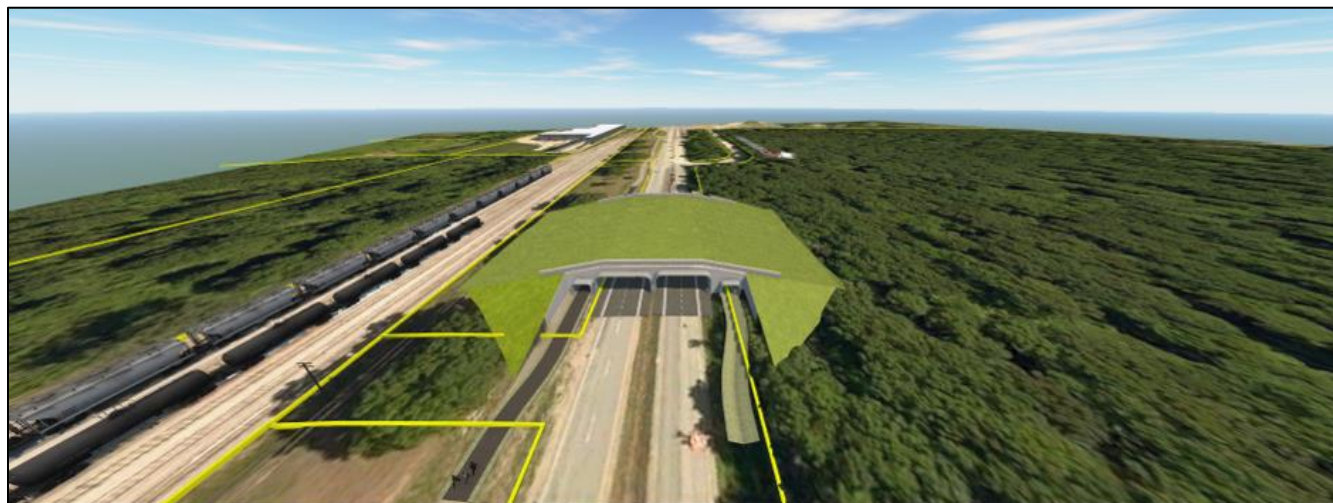
Figure 8-8: Initial Design Option 4 - Wildlife Overpass (4 Span Arch Culvert) – Profile View
