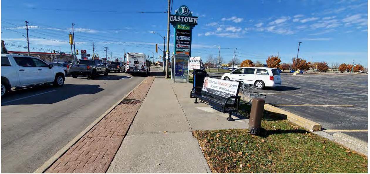
Figure 13 Example of a Near-Side Bus Stop
