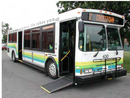
Figure 80 Transit Windsor Accessibility Ramp
