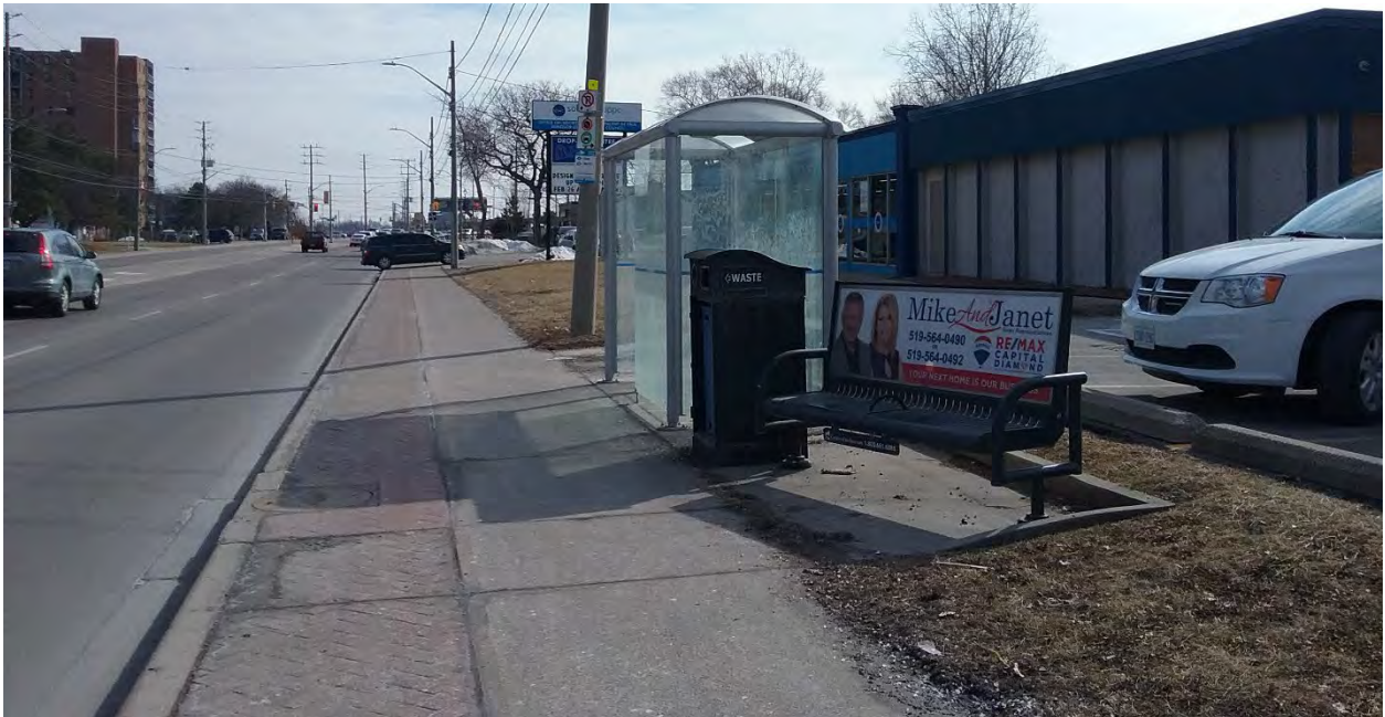
Figure 21 Example of a Mid-Block, In-Lane Bus Stop
