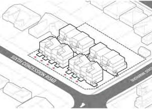
The new development has been designed with a 6.0 metre wide access/driveway from Ducharme Street. The placement of the site access has been optimized to maximize separation from the intersection and also position the driveway to buffer new development, via horizontal plane separation, from existing development and rear yards to the
