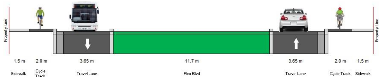
Alternative 6: Cycle Tracks + Flex Boulevard (Representative Cross-Section)
