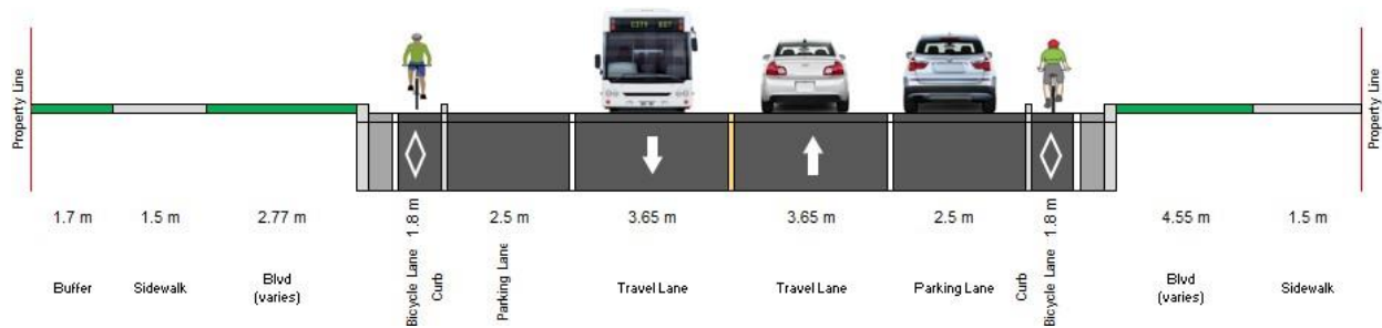
Alternative 1: Physically Protected Bicycle Lanes (Representative Cross-Section)
