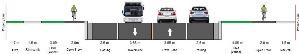
Alternative 3: Cycle Tracks (Representative Cross-Section)
