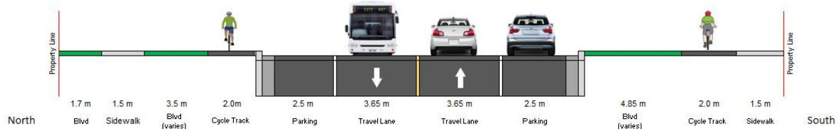
Typical Cross Section - as per Design Plates (August 2020)
