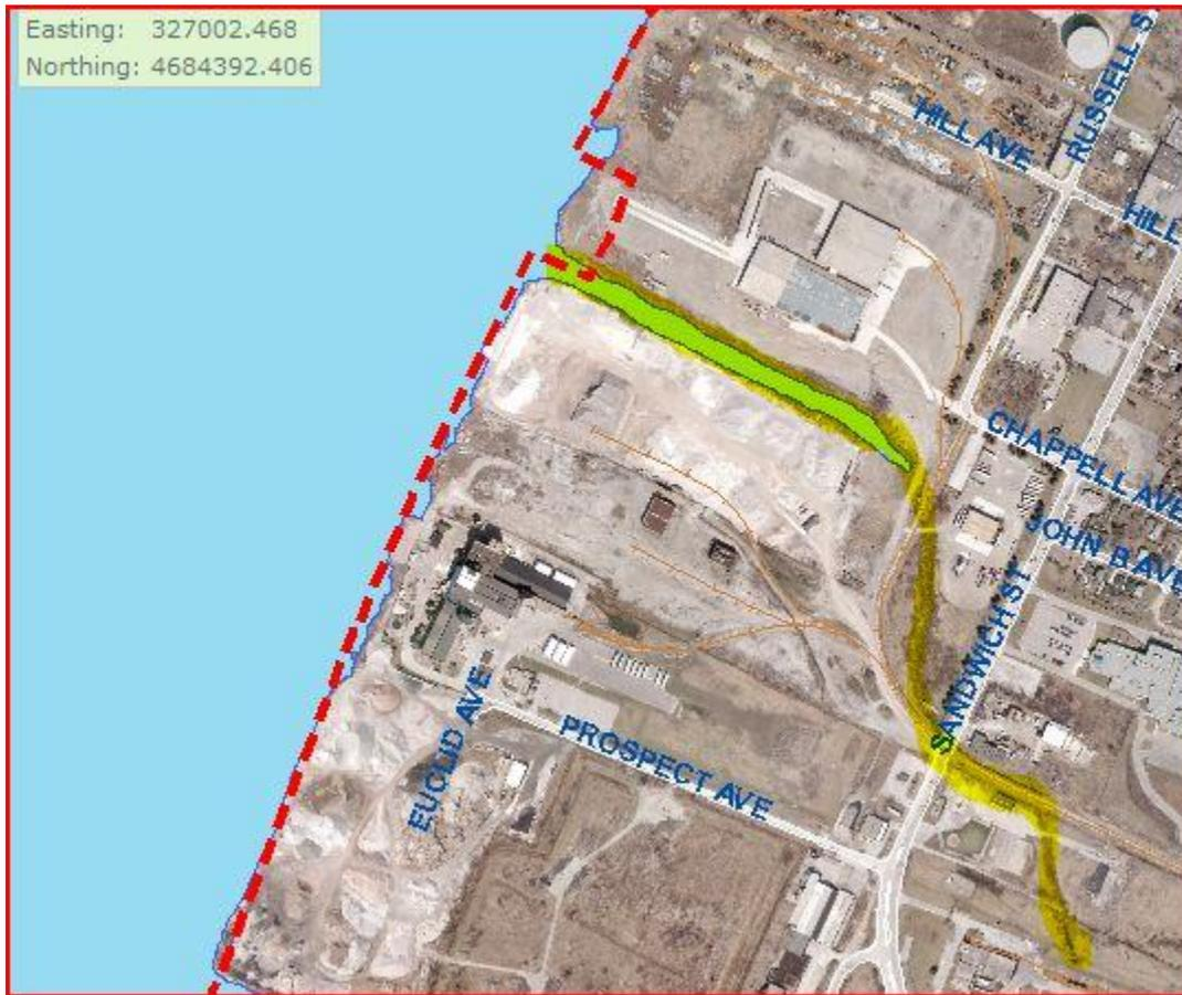
The proposed extension and final connection of the Prince Road storm sewer with the McKee Creek as the final effluent carrier has been determined to result in a detrimental impact on fish habitat (HADD) existing within the lower reach of this Detroit River tributary.
