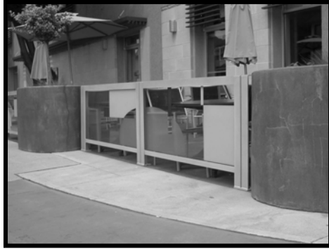
Bolt the post to a stable mass such as a planter
