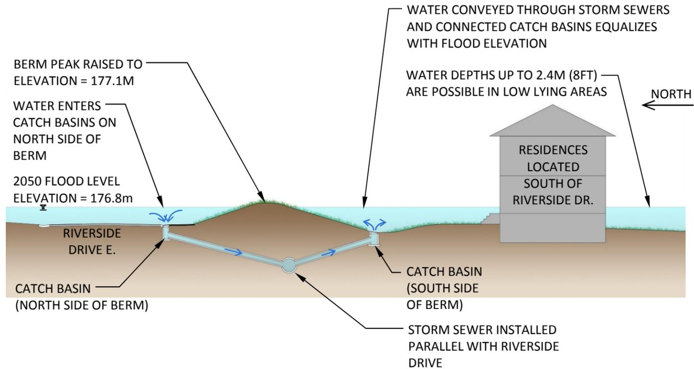
**POTENTIAL SOLUTION:** Modify inlet of catch basin with backflow prevention device (duckbill)
