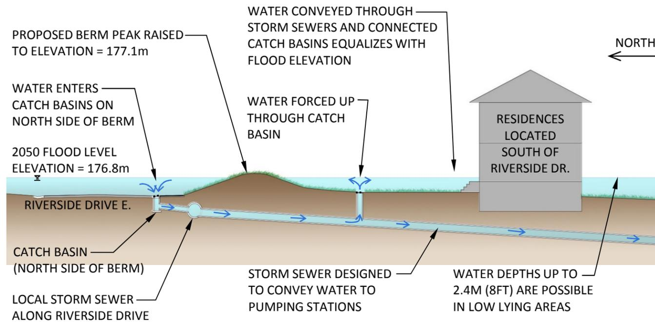
**POTENTIAL SOLUTION:** Install sluice gate inline with storm sewer to prevent flow of water to inland areas during flood conditions
