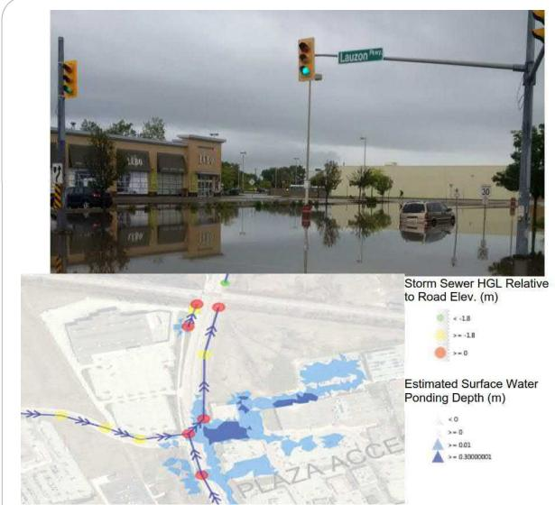
Figure 7.3: Major System – Surface Flooding Calibration Example
