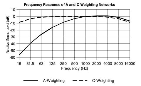
sound pressure signal has been filtered using a frequency weighting that mimics the response of the human ear to loud sound levels. C-weighted sound pressure levels are denoted by the suffix 'C' (ie.
