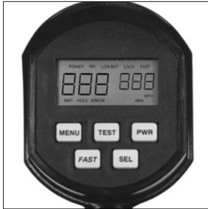
Figure 4.1 Faceplate Display and Control Buttons
