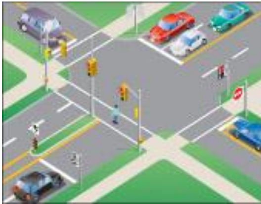
Figure 1: Intersection Pedestrian Signal (source: MTO)
