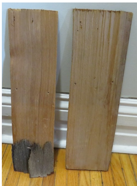
Sample of the new Perfection Cedar Shingles with pieces of the existing cedar roof shingles on bottom left (photo taken June 23, 2023). (The cedar shingles will age to the grey colour.)
