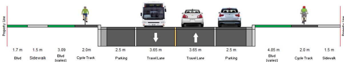
Alternative 3: Cycle Tracks (Representative Cross-Section)
