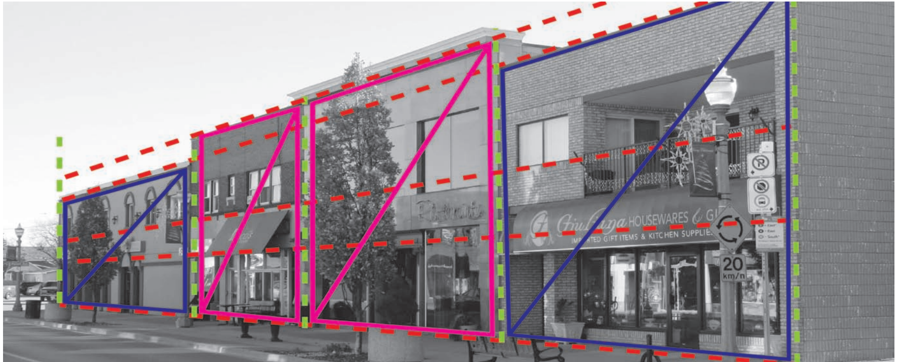
Figure 146. Regulating lines and building proportions identify a consistent pattern along the Erie Street BIA Mainstreet on the south side of Erie Street East from Elsemere Avenue to Parent Avenue.
