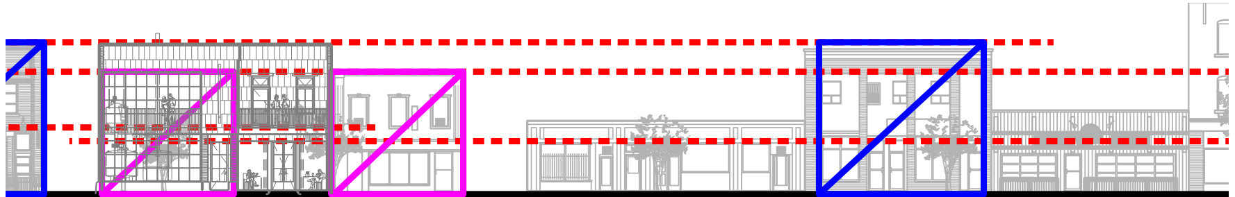
Figure 47. Regulating lines along Sandwich Street, used to inform design of the new microbrewery (Studio g + G Inc. Architect, 2014)
