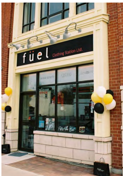
Lighting above signage is directed at the sign and complements the design of the building.
