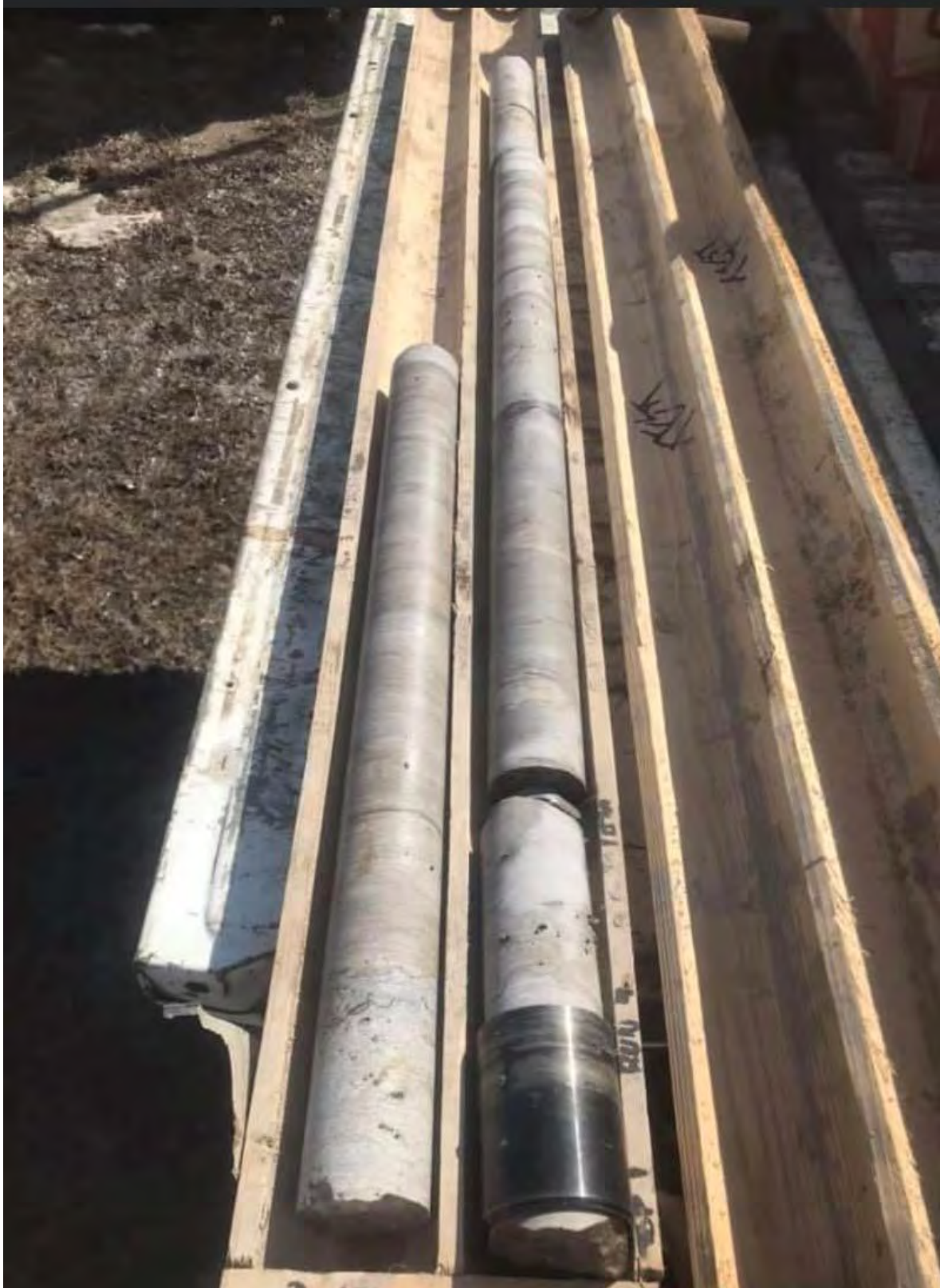
Figure 1: Site Photo of Cores (1-DMT) Run 1: 34.15 m to 36.2 m
