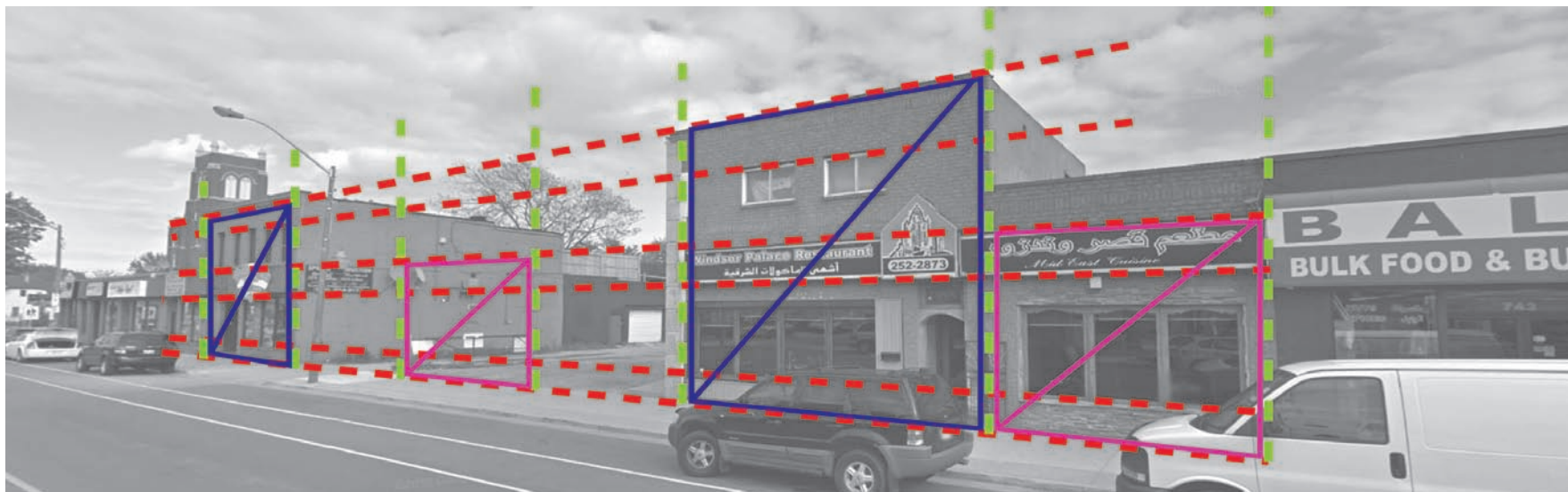
Figure 76. Regulating lines and building proportions identify a pattern along the Wyandotte Towne Centre BIA Mainstreet on the south side from Louis to Marentette Avenue that can be used for infill development.
