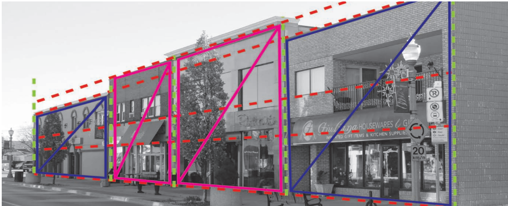
Figure 140. Regulating lines and building proportions identify a consistent pattern along the Erie Street BIA Mainstreet on the south side of Erie Street East from Elsemere Avenue to Parent Avenue.
