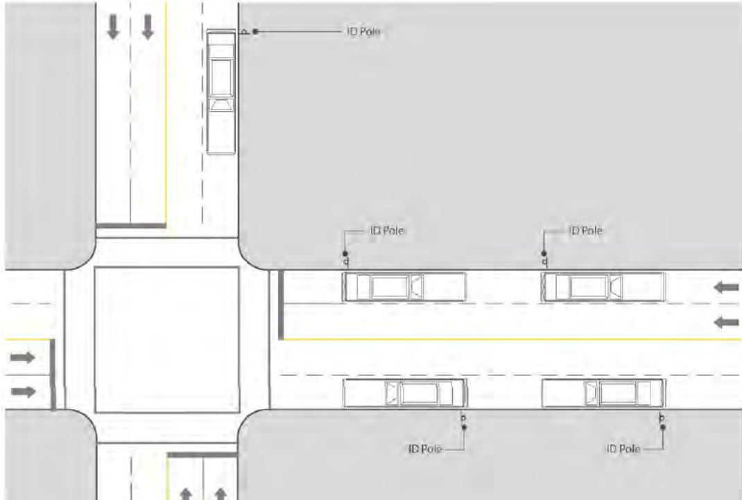
Figure 67 On-Street Terminal Configuration
