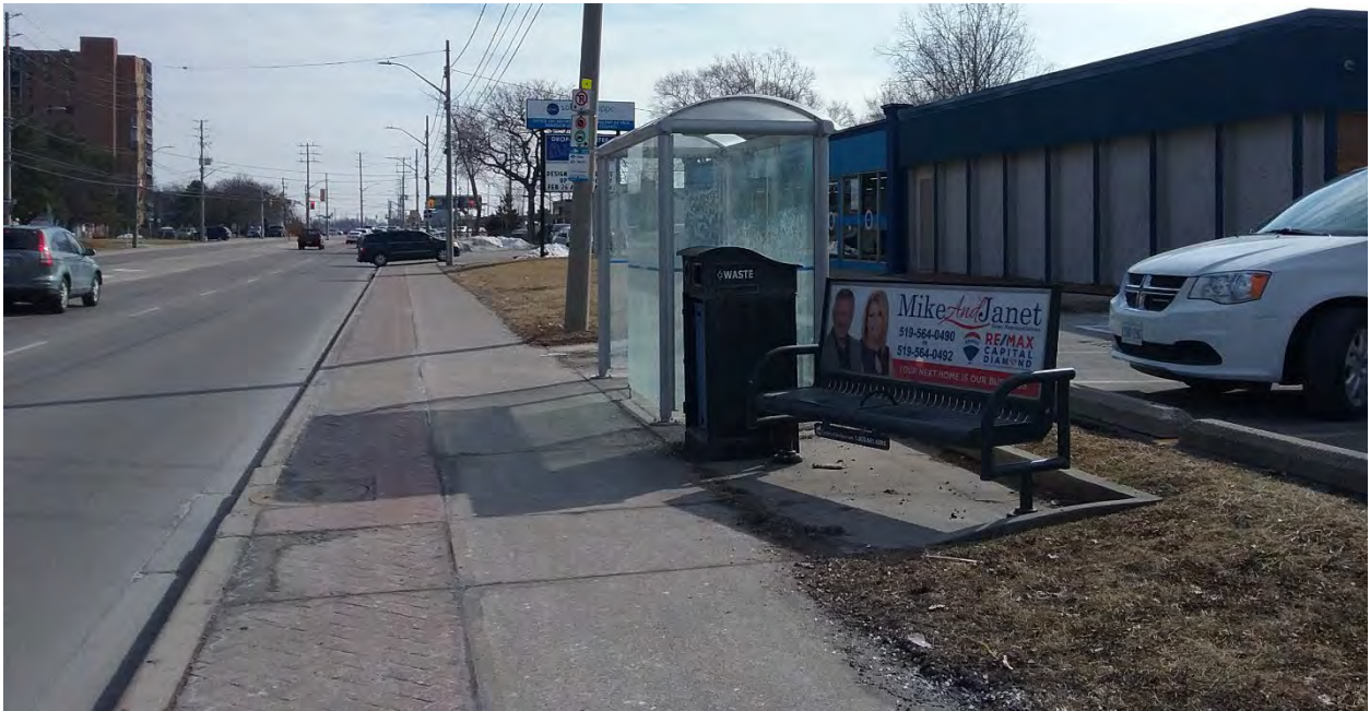
Figure 21 Example of a Mid-Block, In-Lane Bus Stop
