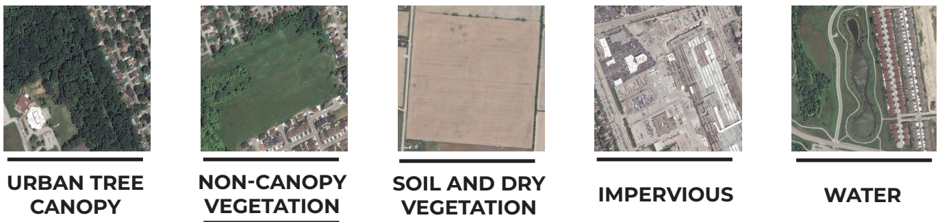
Figure 3. | Five (5) distinct land cover classes were identified in the 2019 tree canopy assessment: urban tree canopy, other non-canopy vegetation, bare soil and dry vegetation, impervious (paved) surfaces, and water.
