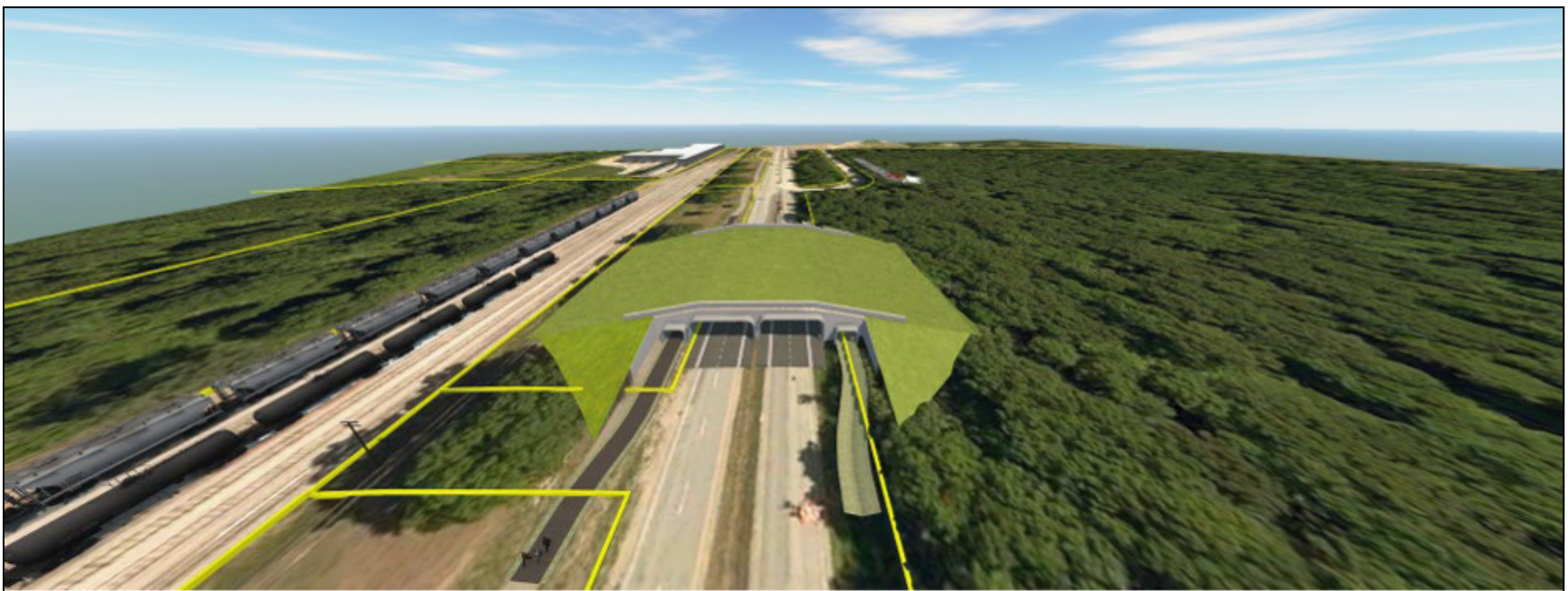
Figure 13: Alternative 4 - Wildlife Overpass (4 Span Arch Culvert)
