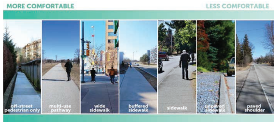
FIGURE 25 - CONTINUUM OF PEDESTRIAN FACILITIES
