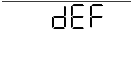
Figure 12. Restoring the Factory Defaults
