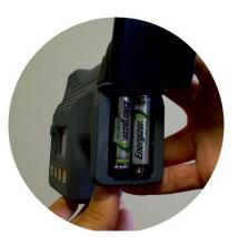
Replace the rubber battery cover and ensure a good seal along the tongue and groove interface.
