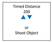
The operator may now enter the reference distance in metres between the two reference objects using the up/down arrows
