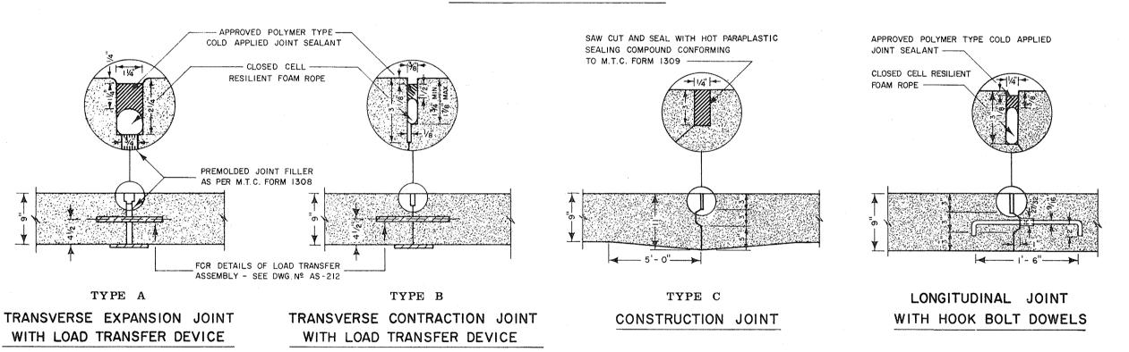
NOTES | ALL PREMOLDED JOINT FILLER, SHALL CONFORM TO M.T.C. FORM 1309.
